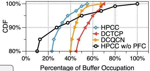
Per-hop flow control (FC) is necessary.
